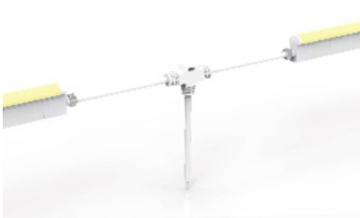
Injection-moulded T-feed Connects two pieces of lights together with a T joint, energized from middle. IP67 Injection-moulded connector. L1 and L2 available in 0.15-0.5m. L3 available in 0.3-3m. Maximum 8 T-feeds in 20m Maximum 4 T-feeds in 10m
